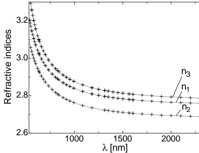
Fig. 4. Principal refractive indices of  $\text{Sn}_2\text{P}_2\text{S}_6$  at  $T = 295 \text{ K}$  in the wavelength range  $550 \dots 2300 \text{ nm}$ . The point signs do not correspond to the error bars ( $\Delta n \approx 2 \cdot 10^{-4}$ ) and for  $n_1$  and  $n_3$  ( $\lambda < 1650 \text{ nm}$ ) data points from two crystals are displayed. The continuous lines correspond to a two-oscillators Sellmeier model with the parameters given in Table 3.
