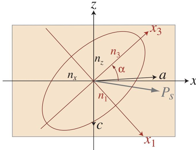
Fig. 1. Position of the indicatrix and spontaneous polarization  $P_S$  in the  $xz$ -plane at room temperature. This is the mirror plane, perpendicular to  $b$  and  $y$ .  $(a, b, c)$  is the crystallographic system (non-orthogonal for monocline crystals),  $(x, y, z)$  is the Cartesian coordinate system, and  $(x_1, x_2, x_3)$  is the dielectric coordinate system.
