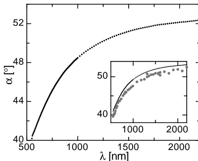
Fig. 2. Measured rotation angle  $\alpha$  of the major axis of the indicatrix to the  $x$ -axis ( $T = 300\text{ K}$ ) Error:  $\pm 0.4^\circ$ . In the inset a comparison is shown with the less precise data calculated from the refractive indices (grey circles).
