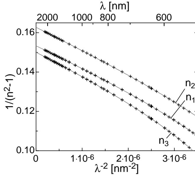
Fig. 5. Principal refractive indices of  $\text{Sn}_2\text{P}_2\text{S}_6$  at  $T = 295\text{ K}$  in the wavelength range  $550 \dots 2300\text{ nm}$ . The coordinate axes are chosen so that a one-oscillator Sellmeier model would appear as a straight line. The continuous lines are from Eq. (6) using the parameters shown in Table 3.
