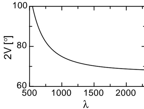
Fig. 3. Angle  $2V$  between the optical axes, calculated from the refractive indices given by Eq. (6) and the parameters in Table 3.
