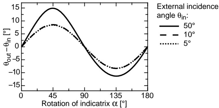
Fig. 7. Calculation of the variation  $\theta_{\text{out}} - \theta_{\text{in}}$  versus the rotation of the indicatrix in the  $xz$ -plane for  $\text{Sn}_2\text{P}_2\text{S}_6$  (Fig. 6).
