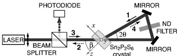
Fig. 4. Experimental setup for the ring-cavity self-pumped phase conjugation with  $\text{Sn}_2\text{P}_2\text{S}_6$ . Without the external loop, input beam 3 was fanned toward the  $+x$  direction. All beams are polarized in the plane of the loop. The transmission grating is written by beam 3 with its self-diffracted beam 4 and by beams 1 and 2 counterpropagating in the loop.
