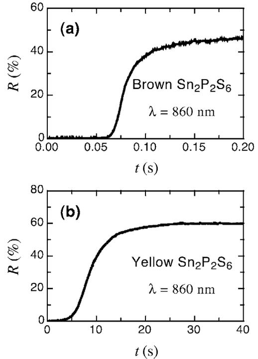
Fig. 5. Time evolution of the phase-conjugate reflectivity  $R$  after input beam 3 was turned on using (a) brown  $\text{Sn}_2\text{P}_2\text{S}_6$  of 2.4 mm thickness and (b) yellow  $\text{Sn}_2\text{P}_2\text{S}_6$  of 9.7 mm thickness. The input beam is at  $\lambda = 860$  nm and has a diameter of 1.2 mm and powers of (a) 30 mW and (b) 90 mW.
