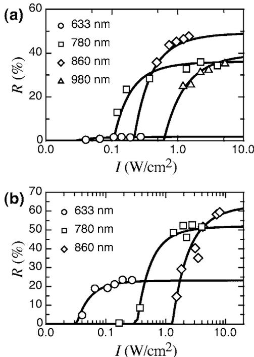
Fig. 7. Measured saturated phase-conjugate reflectivity  $R$  as a function of the incident intensity  $I_3$  using (a) brown  $\text{Sn}_2\text{P}_2\text{S}_6$  and (b) yellow  $\text{Sn}_2\text{P}_2\text{S}_6$ . The solid curves are calculated from Eq. (3) considering additional uniform charge generation included in Eq. (8) with parameters  $\Gamma L$  and  $T_0$  as in Fig. 6 and  $I_\beta$  parameters that correspond best to the measured values (see Table 2).
