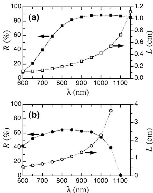
Fig. 11. Optimized phase-conjugate reflectivity  $R$  (left scale) as a function of the light wavelength  $\lambda$  for (a) brown  $\text{Sn}_2\text{P}_2\text{S}_6$  and (b) yellow  $\text{Sn}_2\text{P}_2\text{S}_6$  crystal of the optimal thickness  $L$  (right scale).
