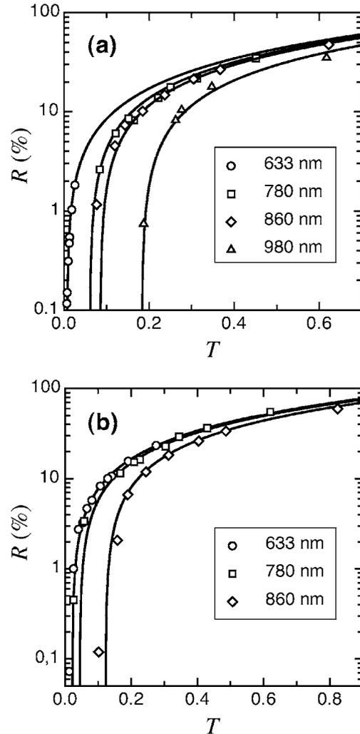
Fig. 6. Measured saturated phase-conjugate reflectivity  $R$  as a function of loop transmission  $T$  using (a) brown Sn<sub>2</sub>P<sub>2</sub>S<sub>6</sub> of 2.4 mm thickness and (b) yellow Sn<sub>2</sub>P<sub>2</sub>S<sub>6</sub> of 9.7 mm thickness. The solid curves are calculated from Eq. (3) with parameters listed in Table 2, where input beam intensities  $I_0$  for this experiment are also given.
