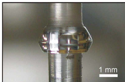
Fig. 1. WGM-resonator made of PMMA with a standard turning lathe.
